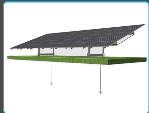
Helical Tie-down Installation
